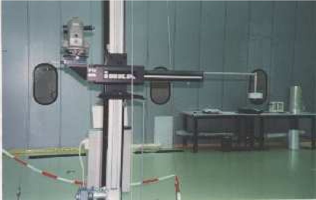
Figure 2.2: ESTEC calibrations: radioactive sources set-up
